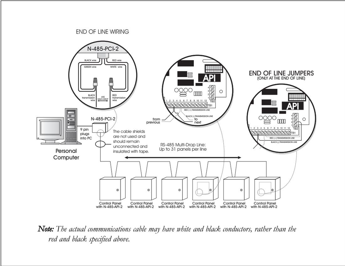
**Configuration 1: N-485-PCI-2 at one end of multi-drop line with panel at other end**
