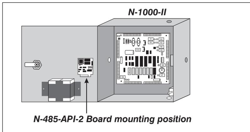
**Note:** Clean the panel surface with an alcohol wipe before attaching the adhesive mounting stand-offs supplied on the printed circuit board.
