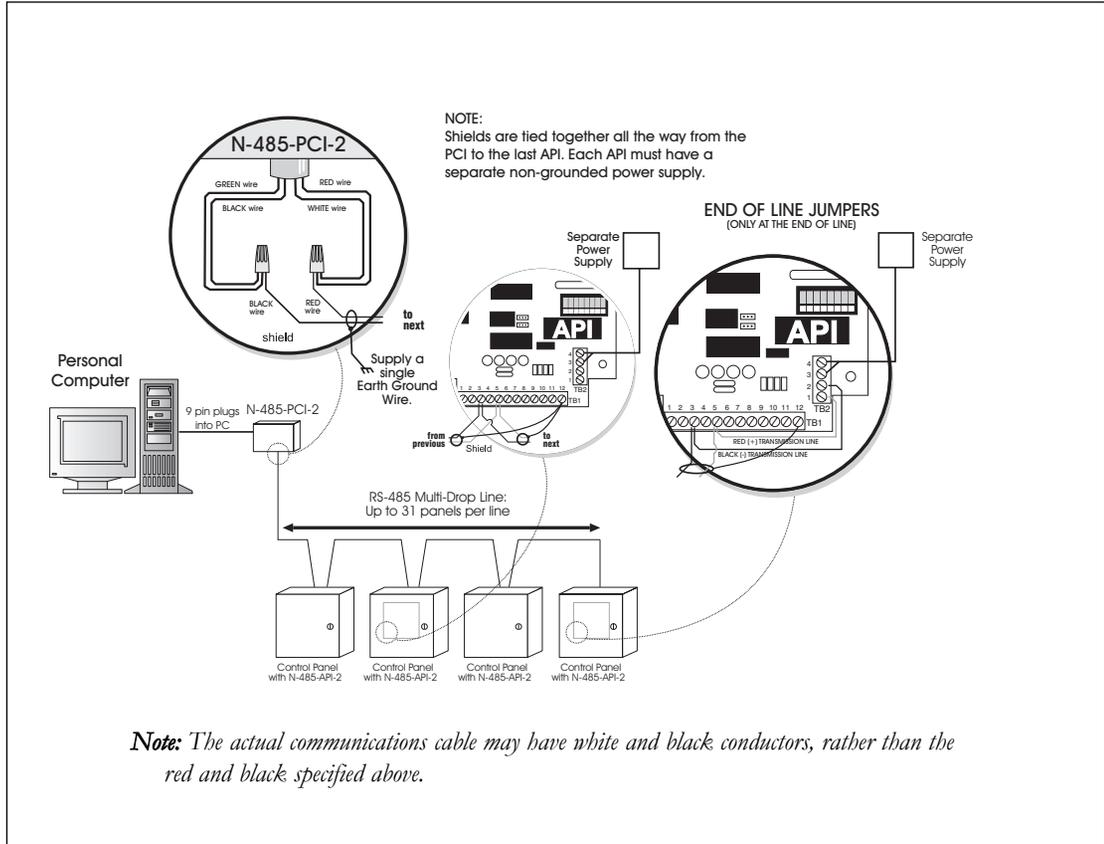
Configuration 4: Special 485 cable wiring for panels in electrically noisy areas
