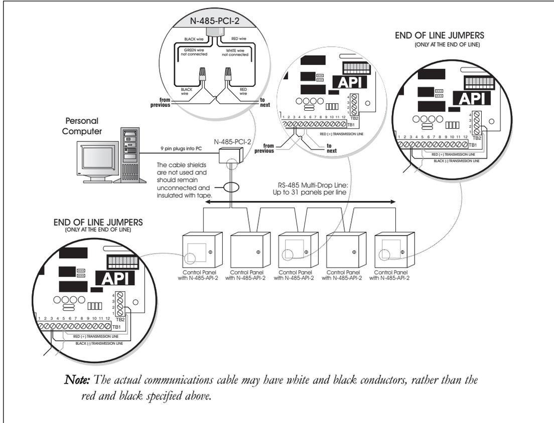
**Configuration 2: Panels at both ends of multi-drop line**
