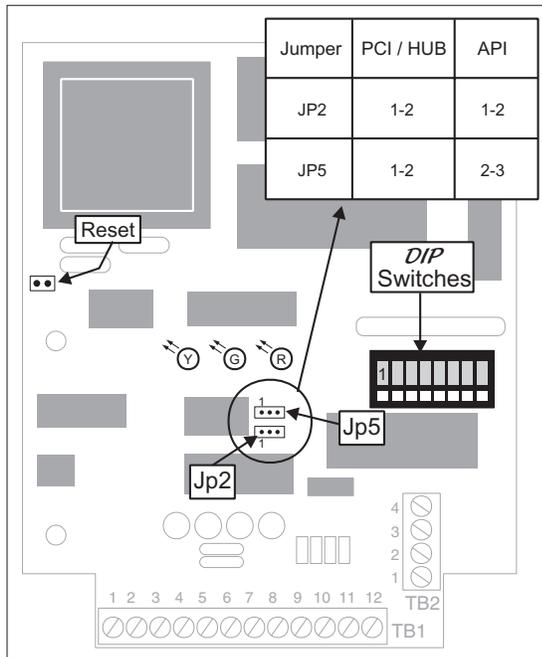
The switches are read at power-up or reset. They must match the settings required by the PC software. If the switch positions are changed while the device is running, the device must be reset or power cycled to have the new switch settings take effect.
